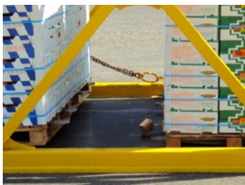
Tines protruding adjacent pallets
