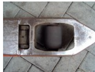
Tine of pallet jack without bogey suspension
