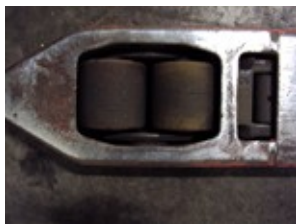
Tine of pallet jack with bogey suspension
